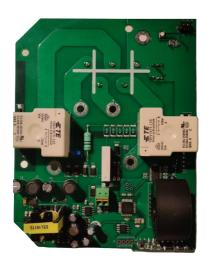
The Deltrix Single Board EV Charging Controller allows integrators to build their own simple but yet safe EV Charging Stations that support from 3.6KW or 7,4KW on a single phase to 11KW on 3 phases and where all components including the relays and DC fault protection are integrated onto a single PCBA.
