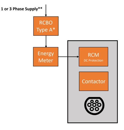
\*A Type B RCBO is not required due to the built-in DC fault protection device (RCM)
